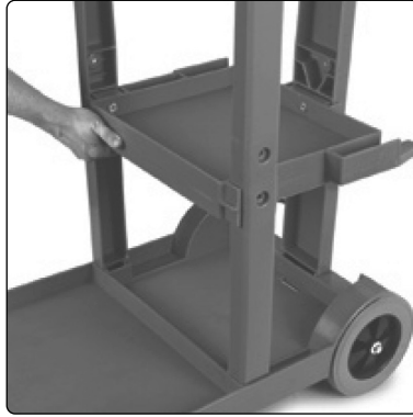
5. Slide middle utility shelf onto uprights as shown. Choose either high or low position and slide post on each side of shelf into corresponding slot on each upright. Tap into place with the mallet.
