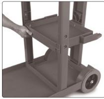
Slide middle utility shelf onto uprights as shown. Choose either high or low position and slide post on each side of shelf into corresponding slot on each upright. Tap into place with the mallet.
