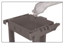
Use 1" bolts inserted from top to lock shelf into place.
