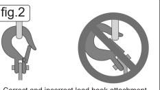
Correct and incorrect load hook attachment
