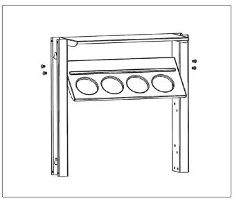
Step 2. Attach the top bottle holder to the left and right stud using the M6 nuts and bolts.
