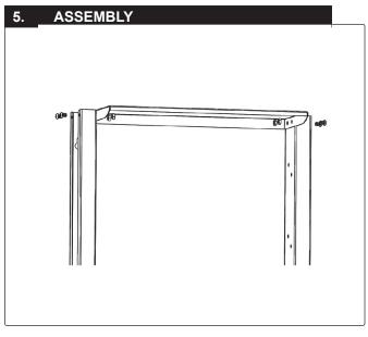
Step 1. Attach shelf to the left and right stud using the M6 nuts and bolts.
