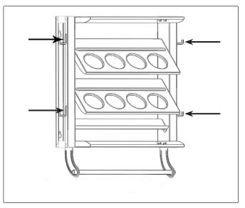
Step 11. Attach the mini hooks to either side as shown.
