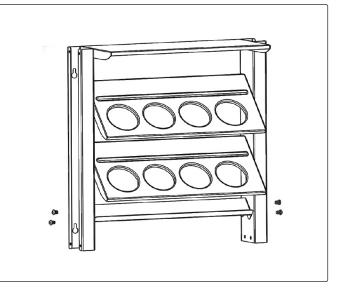
Step 4. Attach the support plate to the left and right stud using the M6 nuts and bolts.
