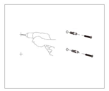
Step 9. Drill the concrete or brick wall with an 8mm drill bit, insert the plastic anchor (wall plugs) into the drilled holes. Screw the M4.8\* 50.8mm mounting screws leaving a 5mm gap for hanging the spray can storage rack.
