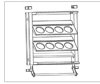
Step 7. Attach the four end caps to each stud as shown in the illustration.
