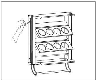
Step 8. Place spray can storage rack up against the wall. Use a spirit level to ensure it is level, using a pencil mark the wall as shown in the illustration.
