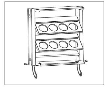
Step 5. Attach shelf and the connecting piece to the left and right stud using the M6 nuts and bolts.
