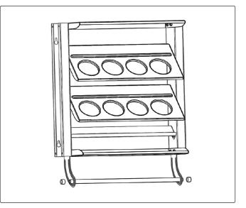
Step 6. Slide the paper towel holder through the connecting piece, then push the plastic end caps on to each end as shown in the illustration.
