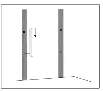
Step 10. Place the spray can storage rack onto the M4.8\* 50.8mm mounting screws, see above illustration. (Weight capacity 100lbs).
