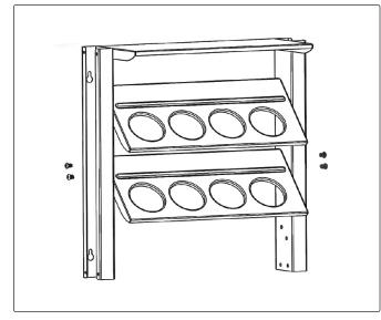
Step 3. Attach the bottom bottle holder to the left and right stud using the M6 nuts and bolts.
