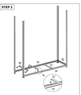
**Step 2:** Slot Brackets 'B' into the bottom of Legs 'D' as shown in the diagram. Slot Braces 'C' into position through the holes provided on Brackets 'A'. NOTE: Flat edges face outwards. Lock rivets to the bottom of the keyhole by tapping the Brackets with a rubber mallet.
