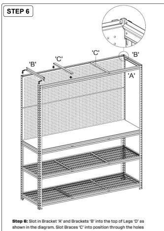
shown in the diagram. Slot Braces 'C' into position through the holes provided. NOTE: Flat edges face outwards. Lock rivets to the bottom of the keyhole by tapping the Brackets with a rubber mallet.
