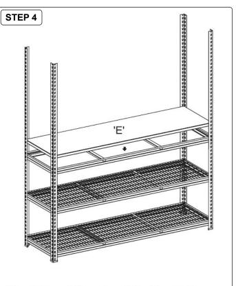
**Step 4:** Repeat Steps 1 and 2 for the middle shelf. Lay the wire shelf and Timber Benchtop 'E' between brackets as shown in the diagram.
