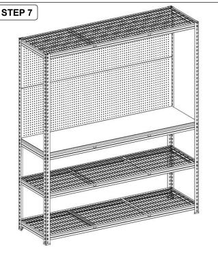
Step 7: Lay the wire shelf between brackets as shown.
