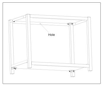
Step 4. To fix on the wall, mark the wall according to the hole which is at the back of top panel, after assembly.
