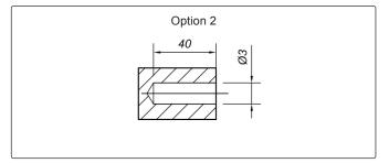
Step 7. To fix the cabinet on to a wooden wall. Mark the wall out before drilling. After the wall has been marked, drill a hole the correct size as illustration.
