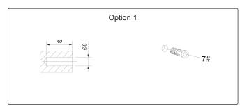
Step 5. To fix the cabinet on to the wall. Mark the wall out before drilling the hole, after the wall has been marked drill a hole the size required as illustration, Insert the wall plug 8\*40.
