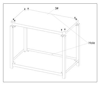
Step 2. Assemble the top panel with screws M6\*12.
