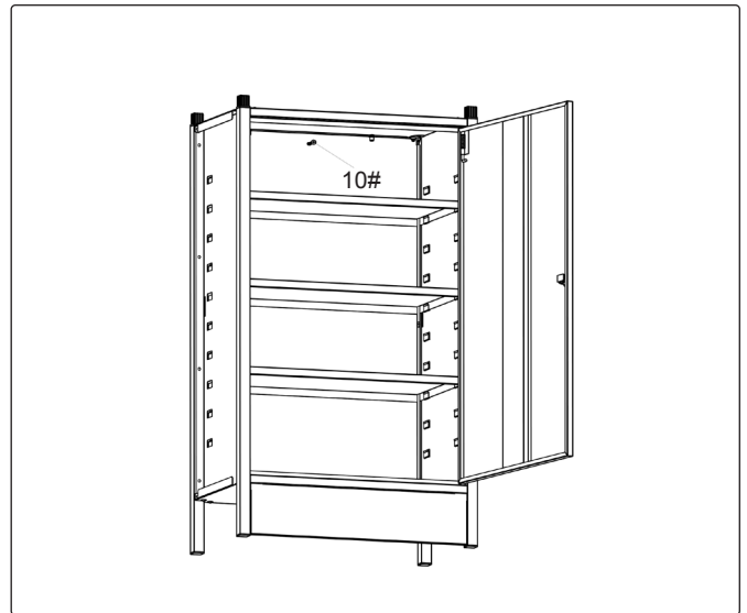
Step 10. Fix to the wall using self-tapping screw ST4.8*30.
