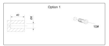
Step 5. To fix the cabinet on the wall. Mark the wall out before drilling the hole, after the wall has been marked drill a hole the size required see above illustration, Insert the wall plug 8\*40 into the drilled hole.
