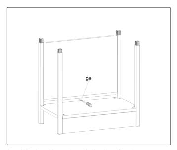
Step 6. Fix the cabinet to the wall using the self-tapping screw ST4.8\*30.
