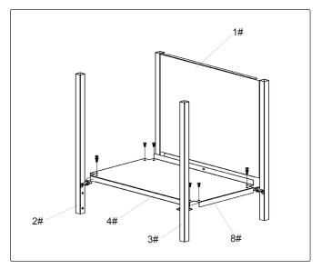
Step 1. Assemble the uprights, back board and the bottom panel with screw M6\*12 as shown.
