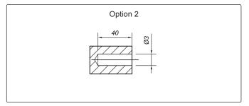
Step 7. To fix the cabinet on to a wooden wall. Mark the wall out before drilling. After the wall has been marked, drill a hole the correct size.
