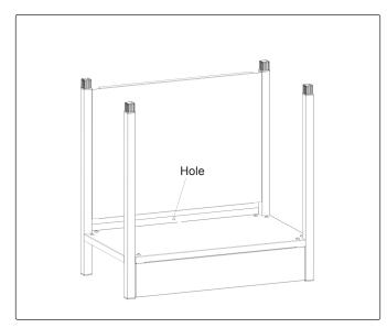
Step 4. To fix on the wall, mark the wall according to the hole which is at the back of the bottom board.
