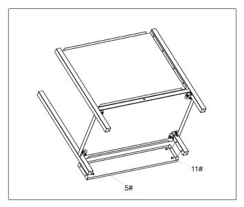
Step 2. Assemble the skirting board with screws M4\*10.
