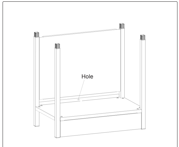
Step 4. To fix on the wall, mark the wall according to the hole which is at the back of the bottom board.
