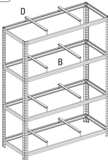
Slot Braces (Part D) into position through the holes provided on the Long Beams (Part B).
