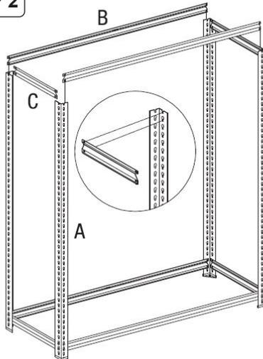
Fasten Short Beams (Part C) to the top of the Angle Posts (Part A) as shown, followed by Long Beams (Part B) to opposing keyholes to form the frame. **NOTE:** Flat edges face outwards. Lock rivets to the bottom of the keyhole by tapping the Beams with a Rubber Mallet.
