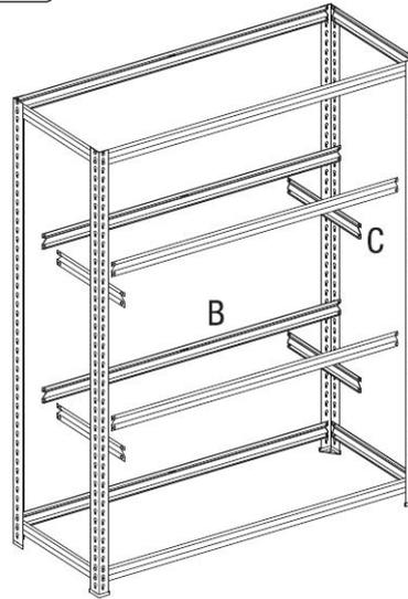
Assemble remaining Short Beams (Part C) and Long Beams (Part B) to your desired shelf height. As before, lock rivets to the bottom of the keyhole by tapping the Beams with a rubber mallet.
