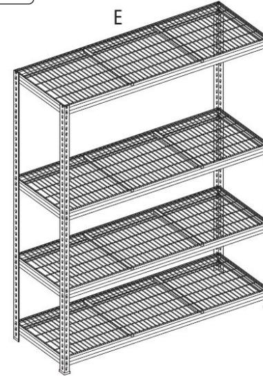
Lay the Wire Shelving (Part E) between the Beams as shown.
