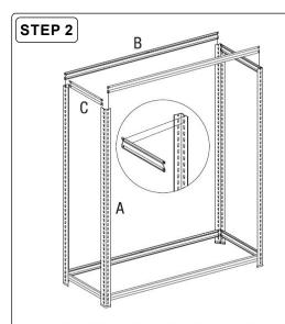
Fasten Short Beams (Part C) to the top of the Angle Posts (Part A) as shown, followed by Long Beams (Part B) to opposing keyholes to form the frame. NOTE: Flat edges face outwards. Lock rivets to the bottom of the keyhole by tapping the Beams with a Rubber Mallet.
