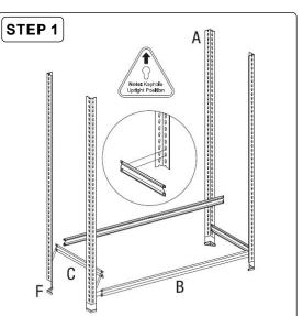
Add Rubber Feet (Part F) to bottom of Angle Posts (Part A). Slot Short Beams (Part C) to the bottom of the Angle Posts (Part A) as shown, followed by Long Beams (Part B) to opposing keyholes (in holes 2nd and 3rd from bottom). NOTE: Flat edges face outwards. Lock rivets to the bottom of the keyhole by tapping the Beams with a rubber mallet.
