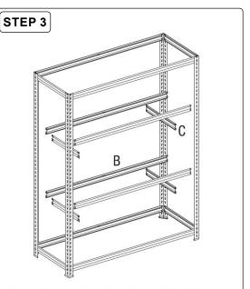
Assemble remaining Short Beams (Part C) and Long Beams (Part B) to your desired shelf height. As before, lock rivets to the bottom of the keyhole by tapping the Beams with a rubber mallet.
