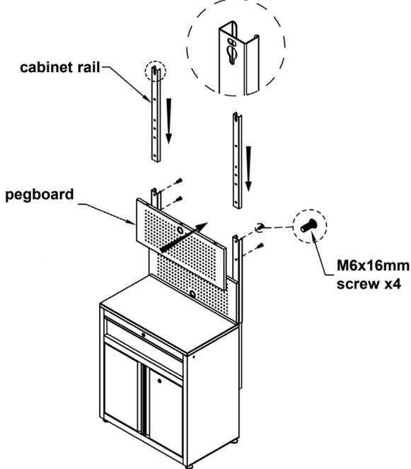
**STEP 5:** Screw two M6x16mm screws, into the back of the top cabinet, leaving a 0.8cm gap. Do not tighten bolts fully. Hang the wall cabinet on the top of the posts, then fully tighten the screws. Attach the bottom of the wall cabinet to the posts using another 2x M6x16mm screws.
