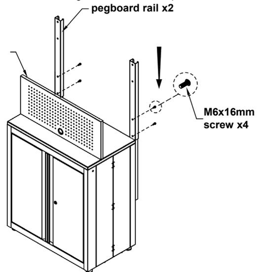
**STEP 8:** Slide 2 cabinet rails onto the pegboard rails. Make sure to leave enough room at the top for the wall cabinet. Place one pegboard on the front, making sure the grommet hole is on the top. Attach using 2x M6x16mm screws per rail.
