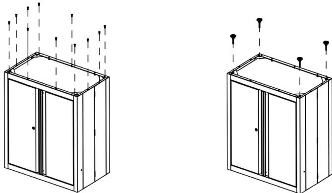
**STEP 4:** Attach the worktop to the cabinet using 4x M6x16mm screws.
