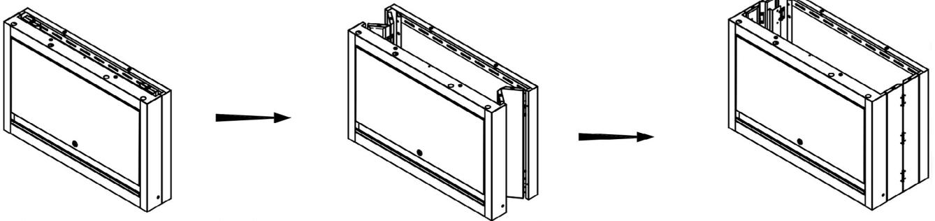
**STEP 2:** attach the top panel using 8x M6x16mm screws.
