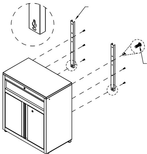
**STEP 3: Slide 2x peg board rails fully onto the cabinet posts. Place one pegboard on the front, making sure the grommet hole is on the bottom. Attach using 2x M6x16mm screws per rail.**
