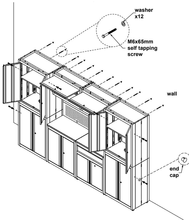
**STEP 12:** Attach the modular storage kit to the wall using twelve M6x65mm tapping screws and washers insert through wall studs. Insert the 6 end cups on the side panels of the cabinets.
