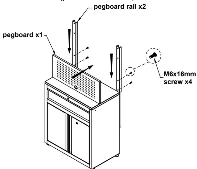
**STEP 4:** Slide 2 cabinet rails onto the pegboard rails. Ensure there is enough room at the top for the wall cabinet. Attach 2 cabinet rails using 2x M6x16mm screws per rail. Attach second pegboard, ensure grommet hole is at the top.
