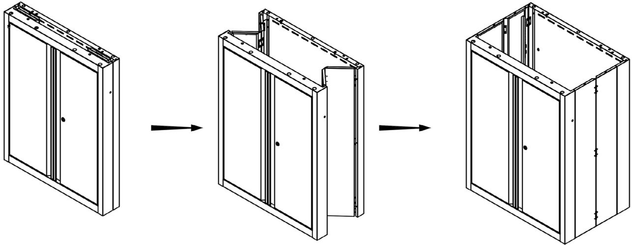
**STEP 2 TOP CABINET:** Attach the top panel using 8x M6x16mm hex socket head screws.
