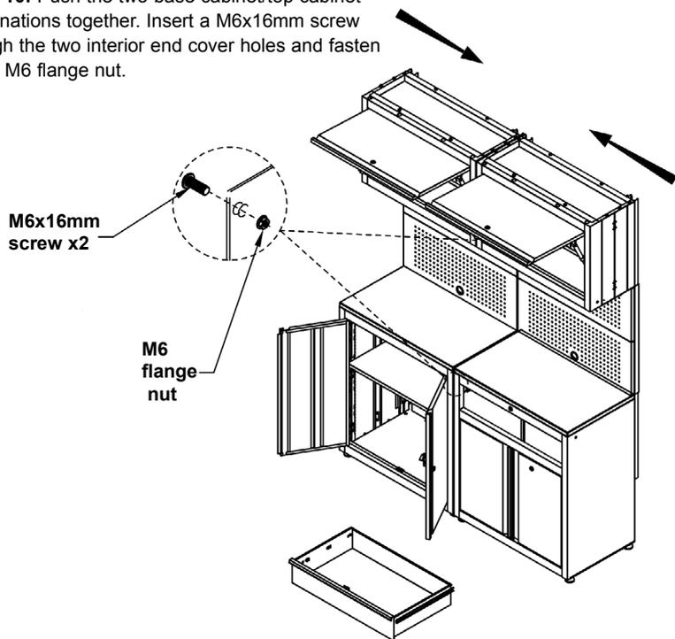
**STEP 11:** Push a stackable cabinet combination towards either side of the base cabinet/top cabinet combination. Insert a M6x16mm screw through the two interior end cover holes and secure with a M6 flange nut.
