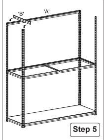
Fix brackets 'B' at the very top allowing room for the MDF board to sit flush against the legs. Repeat with brackets 'A'.
