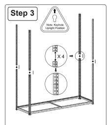
Place MDF board on bottom shelf to minimise buckling. Join the upper legs to the lower legs with the connector pins. Note upright position. Note: The legs are designed to sit directly on top of each other – don't overlap them. Handy Hint: Flathead screwdriver may be used to tap in connector pins.
