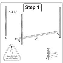
Allow one keyhole free between the foot cap and the shelving bracket.
