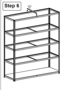
Apply remaining brackets as above to desired height. Ensure that braces 'C' are fixed to all shelves
