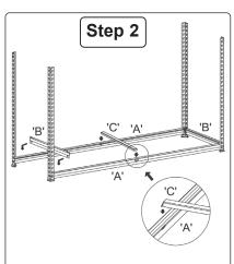
Use shelf bracket 'B' for the side brackets using the shelf bracket from Step 1 as a guide for height. Allow 1 keyhole free from the ground as shown in the diagram. Use same shelving brackets for opposing sides as shown in the diagram. Place brace 'C' as shown.
