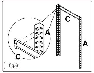
5.4. See Fig.6. Now make up an upper end frame by connecting two angle posts together at the top with a short step beam (C). Tap the beam at either end to ensure that the tabs are properly seated in the slots. Make up a second upper end frame using the remaining two angle posts and a short step beam.
