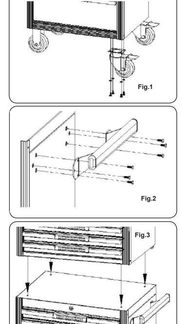
**3.2** Fasten the handle with the screws provided as fig.2.
