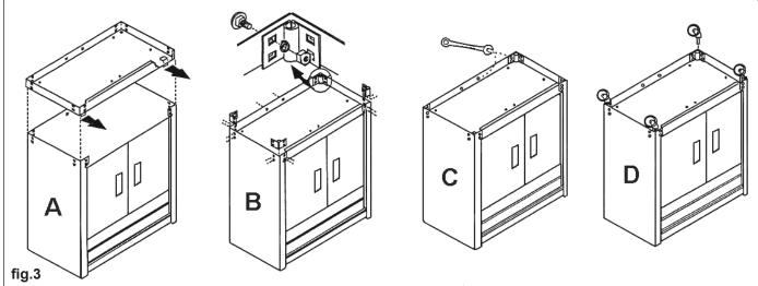
3.3 Turn the rollcab upside down and place the base into position as shown in fig.3A.
