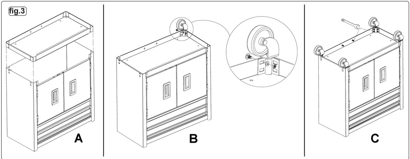
4.3. Turn the rollcab upside down and place the base into position as shown in fig.3A.
