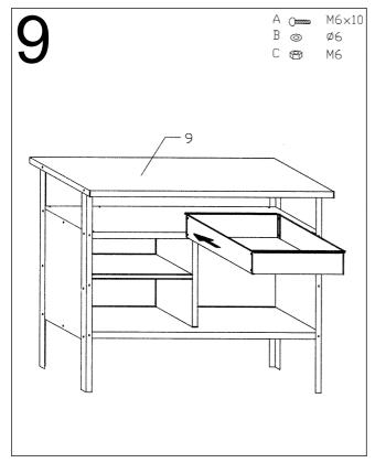
**STEP 9.** When the work surface is secure slide the drawer into the slots that were fixed to the underside of the work surface at step 6.
