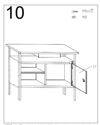
**STEP 10**. The righthand side of the lower storage area is going to be made into a cupboard, to do this take the cupboard door (17) and fix to the top and bottom panels of the lower storage area, as shown in the diagram above.
