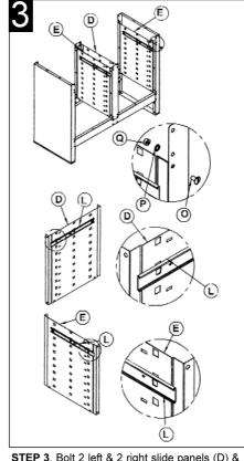
STEP 3. Bolt 2 left & 2 right slide panels (D) & (E) into position, only bolt at front of Work Bench using 8 bolts (O), 8 lock washers (P), and 8 nuts (Q). Fix 1 left hand female slide (L), at top onto each slide panel (D) and 1 right hand female slide (L), onto each slide panel (E) Refer to Diagram 11 on how to fit slides.
