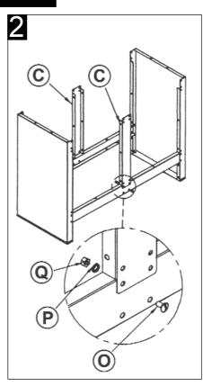
**STEP 2**. Bolt the two centre supports (C) to the front and back crossrails respectively using 4 bolts (O), 4 lock washers (P), and 4 nuts (Q).
