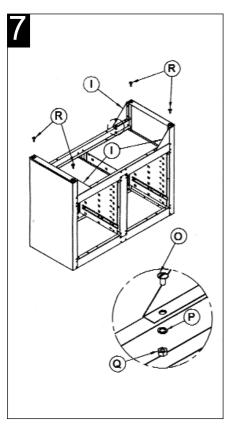
STEP 7. Screw in the four adjustable leg levellers (R). Bolt the four corner braces (I) into position using 16 bolts (O), 16 lock washers (P), and 16 nuts (Q)
