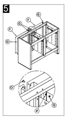
STEP 5. Take two draw stops (G) and one back panel (F) and bolt them to the back of the cabinet with the draw stops between the panel and the cabinet. Repeat procedure with the other back panel and 2 draw stops. Use 8 bolts (O), 8 lock washers (P), and 8 nuts (Q).
