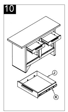
STEP 10. Attach a left hand female slide (K) to left hand side of each draw and a right hand female slide (K) to the right hand side of each draw (see diagram 11). Engage each draw onto the protruding male slides and push fully home, then open the draw to check that it is retained.
