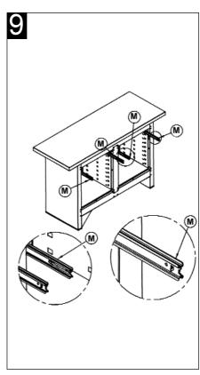
STEP 9. Take the 4 male slide components (M) and slide 2 onto the female slides on the left of the draw compartment and 2 onto the female slides on the right hand side of the draw compartment. Push them fully in to engage them, then pull them out to the stop point.
