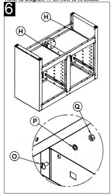
STEP 6. Turn the cabinet upside down and bolt the two shelf components (H) into position at the bottom of the unit using 8 bolts (O), 8 lock washers(P), and 8 nuts (Q).
