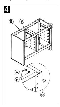
STEP 4. Take two crossrails (B) and bolt them to the cabinet sides (A) and centre supports (C) using 12 bolts (O), 12 lock washers (P), and 12 nuts (Q).
