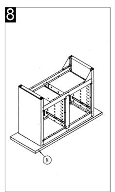
STEP 8. Place the wooden top (N) face down on a flat, clean, smooth surface. Position the cabinet upside down on the wooden top and mark the hole locations on the top. Move the cabinet to one side and drill 5/32" diameter x 1/2" deep holes in the top. DO NOT DRILL DEEPER THAN 1/2". Attach frame to top with the 4 hex head screws (S).
