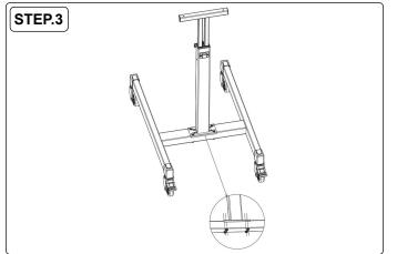
3. Place the support frame assembly on the base as shown, paying attention to the front and rear orientation. Secure with bolt, flat washer and anti-loose nut, using the wrench provided.
