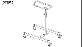
5. Install the upper support tube assembly on the support frame assembly as shown. Secure with 2 hexagonal screws, flat washers and anti-loose nuts, using the wrench provided.
