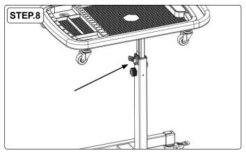
8. To adjust the height, first unlock the clip to the left of the support frame. Loosen the hand screw counterclockwise.
