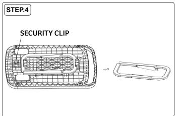
4. Ensure the security clip is 'open' as shown above. Push the upper support frame assembly horizontally to the left and remove it from the tool tray assembly.
