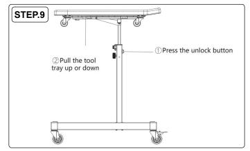
9. Press the unlock button and pull the tool tray up/down to adjust the height.
