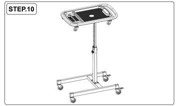
10. After confirming the height adjustment, the "click sound" indicates that the adjustment is completed. Press the clip to the right, and finally tighten the screw clockwise to secure the tray in position.
