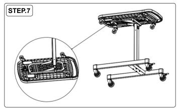
7. Install the tool tray assembly on the upper support tube as shown. Rotate the security clip to the 'closed' position to secure the tool tray into position.
