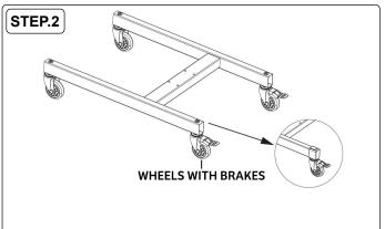
2. Pass the tube nut through the square tube hole of the underframe. Fit the 3" wheels, and tighten with a wrench. Ensure the wheels with brakes are installed at the correct end of the underframe. Insert the plugs back onto the underframe.
