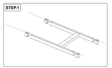
1. Remove the plugs from both sides of the underframe. Leave them off until the wheels have been installed.
