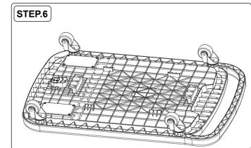
6. Install the 2" wheels in the screw holes of the tool tray as shown. Tighten with the wrench provided.
