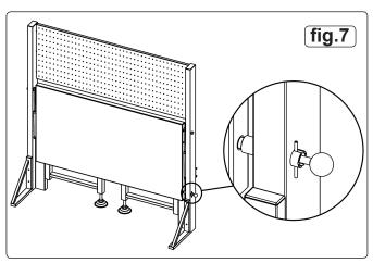
3.8 To stow table remove the bolts securing the worktable to the folding legs. Adjust the feet, to allow movement of the folding legs. Fold the legs back and push the worktable down into the vertical position. Twist the lock pin and ensure it locks the worktable in place.
