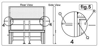
Attach the worktable to the two main support legs using the 3.4 two large bolts (O) and washers (Q). Secure with nut (R).
