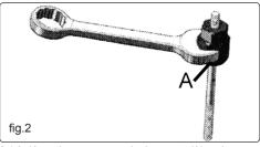
2.1.3 Keep the spanner on the lower nut (A) and unscrew the stud
