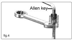
2.2.3 When the stud is screwed in securely, loosen the allen screw on the top of the nut with the allen key provided. The insert nut will now be able to be removed without loosening the stud.
