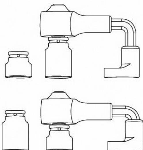
90° Reaction Bar can be adjusted to use with normal and deep socket.
