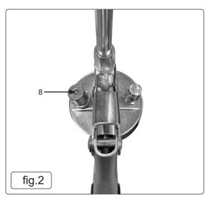
□ WARNING! An empty grease cartridge or grease may be under pressure from the spring in the barrel, use caution when removing it.
