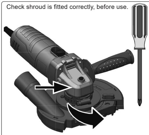
5.1. Connect to vacuum extraction. Risk assess the cutting task to be performed. Perform a run up test and operation of the shroud before commencing work to ensure all parts are correctly aligned.
