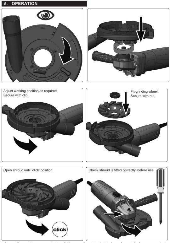
Select grinder ring spacer and fit onto grinder. Fit dust shroud onto grinder.
