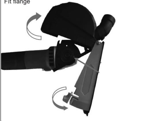
Fit flange nut, tighten
