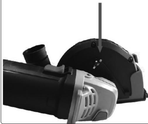
Pass grinder through shroud assembly.
