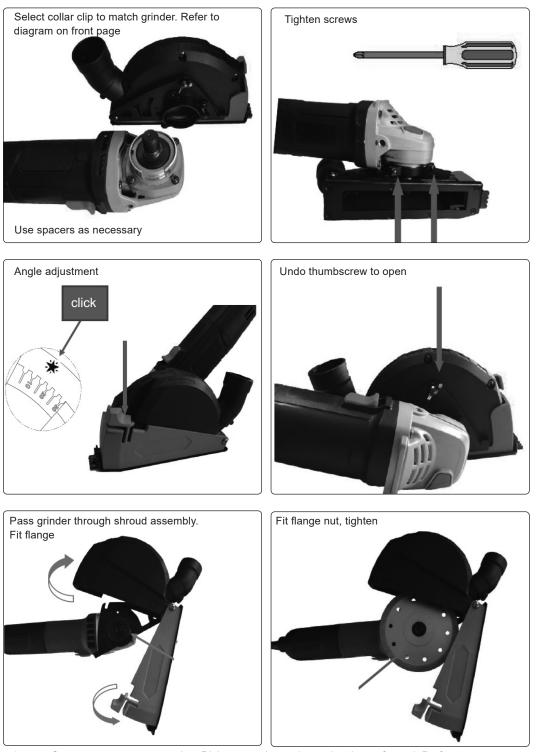
5.1. Connect to vacuum extraction. Risk assess the cutting task to be performed. Perform a run up test and operation of the shroud before commencing work to ensure all parts are correctly aligned.
