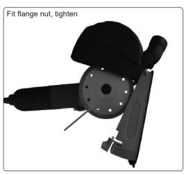
5.1. Connect to vacuum extraction. Risk assess the cutting task to be performed. Perform a run up test and operation of the shroud before commencing work to ensure all parts are correctly aligned.
