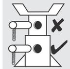
Fit pin through both the stand collar and the centre tube
