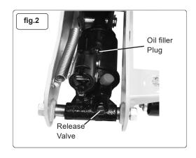
Open the release valve and, by stepping on the saddle, force the arm to lower as rapidly as possible. Repeat this operation three or four times.
