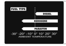
Although our heaters operate with diesel fuel, when the temperatures are below 0°C, diesel additives are required to maintain the diesel's viscosity. Typically diesel can cloud in freezing conditions and will start to gel. You will need additives for your fuel in these conditions.
