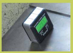
Its tough alloy rim has a magnetic base so will attach itself happily to steeply tilted, vertical steel or cast-iron surfaces
