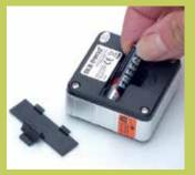
Powered by a single AAA battery (included), this is inserted in the rear compartment
