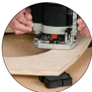
Routing with bottom clearance. Simply position blocks in corners.
