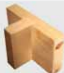
Through housing joint using tenon slide template.
