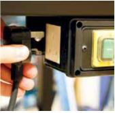
The router is controlled by plugging it into the NVR switch provided
