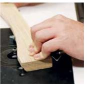
You can see the principle here, providing a pivot point to introduce the work to the cutter
