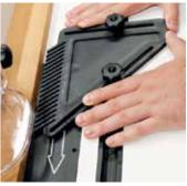
Adjustable featherboards are supplied for both vertical and horizontal control
