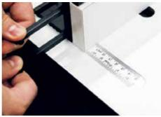
These two rods slide behind the outfeed fence to pack it off for planing functions
