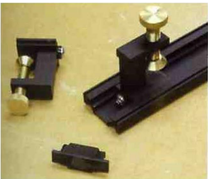
The bespoke clamps slide into the underside of the extrusion
