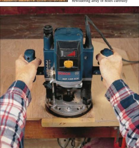
► The Unibase with its centring pin and a dummy guidebush in place
