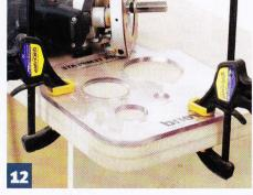
the pivot point is mounted on a plate that fits underneath the router, so it can be used to cut circles down to 25mm in diameter...
