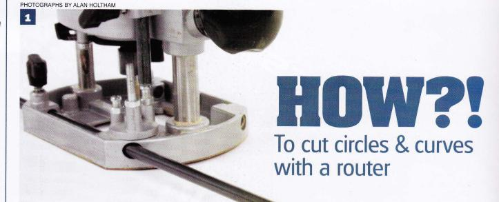
The router is ideal for cutting and moulding accurate circles and curves, writes Alan Holtham. If they have a constant radius the curves can be cut by pivoting the router about a fixed point using an adjustable trammel. Most routers can be used with trammels, both for cutting the initial shape and for applying a decorative edge profile, or the shape can be cut first using a trammel and then the decorative moulding applied conventionally using a bearing-guided cutter.
