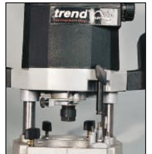
▼ The spindle lock and depth stop work well
