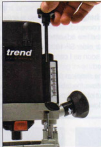
The spindle lock makes it easy to change cutters
