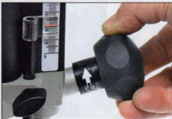
The right side handle operates as the plunge lock
