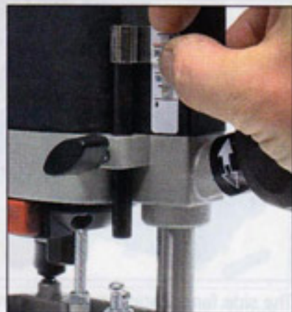
The depth stop is the ubiquitous rod type
