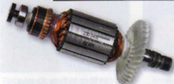
The armature shows little sign of needing balancing
