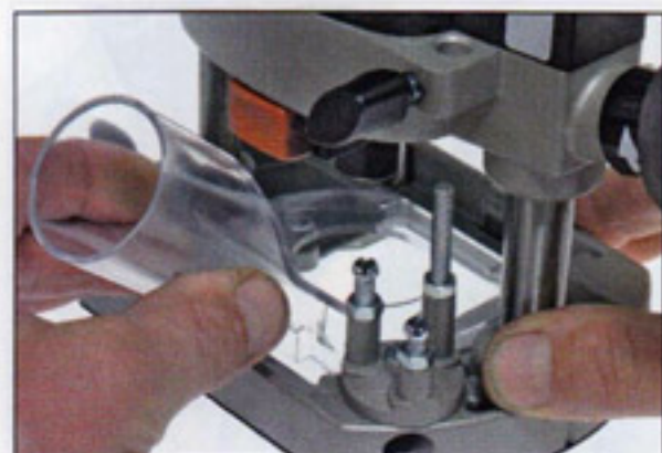
The plastic hood can fit on either side of the base
