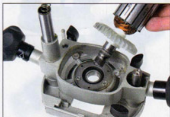
The main bearing is more substantial than the others
