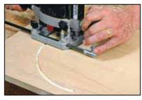
Using the beam trammel bar to make circles and arcs.
