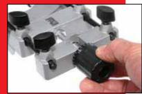
Adjusting the fence using the microfine fence adjuste
