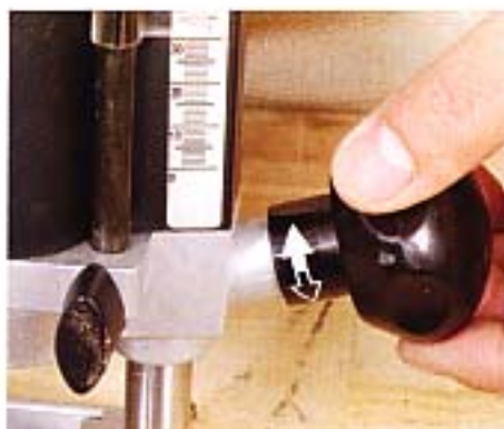
To plunge you twist the handle, push the machine downwards and twist the knob again to lock
