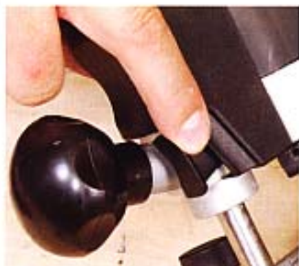
To activate the router you slide out a lever switch alongside the handle with your thumb
