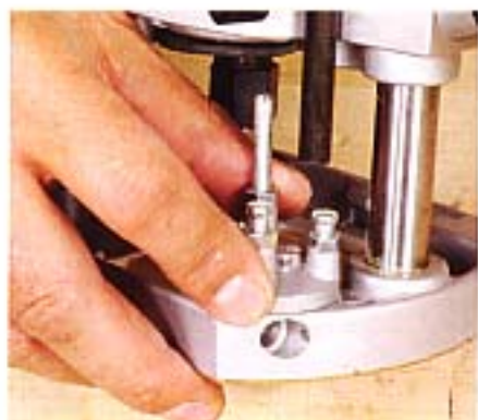
A basic three-way turret is fitted, although each of the stops can be adjusted with a screwdriver
