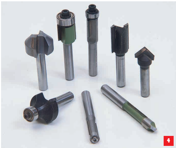
Selection of cutters suitable for use with the T2. Maximum diameter is 23mm
