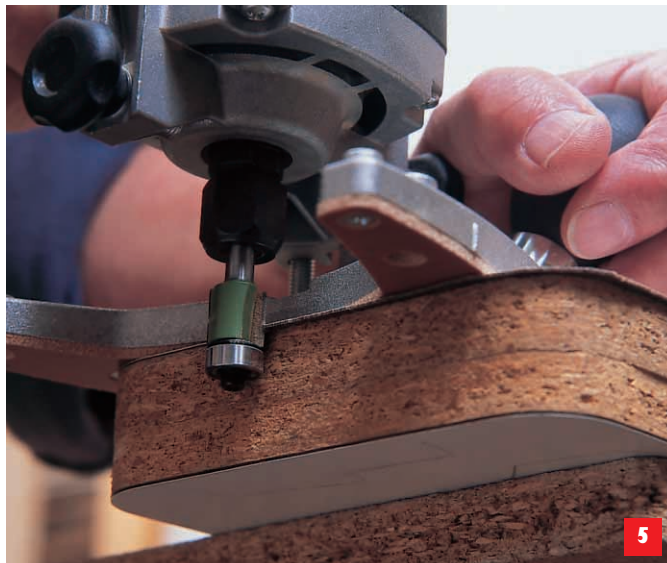
Router stand with laminate overhang being trimmed with bearing-guided flush trimmer fitted
