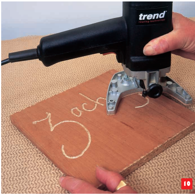
First shot at lettering with the T2, fitted with a V-grooving cutter
