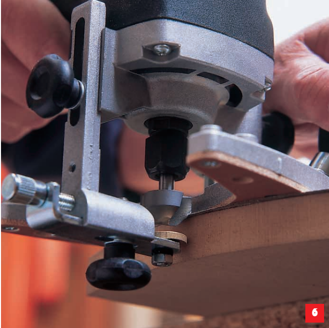
Plastic overhang on wall plaque being trimmed to 45° with combi-trimmer and roller copy follower
