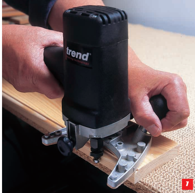
Moulding the edge of a board with bearing-guided round over cutter
