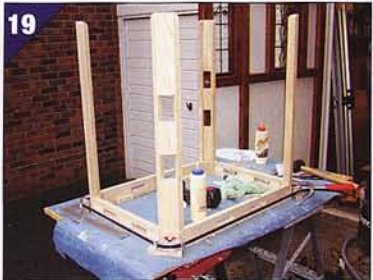
Check that the assembly is square
