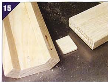
15 Cut the loose tenons and check the fit
