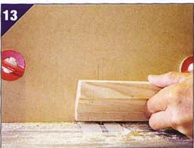
Lower each leg onto the router cutter, using the marks to give the correct position and length
