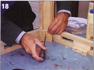
Attach the first leg support
