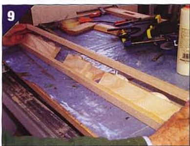
Set up the router and the table to cut the mortises for the loose tenons
