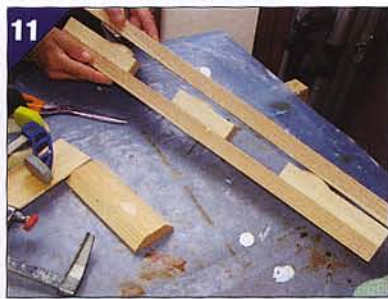
Repeat with each rail. Make progressive cuts to the correct depth
