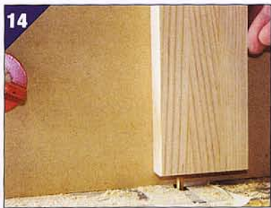
Repeat with each rail. Make progressive cuts to the correct depth
