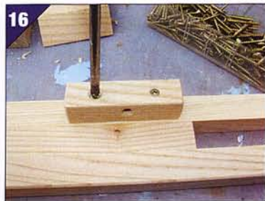
16 Fix the rail to the table top attaching blocks to the top of the rails
