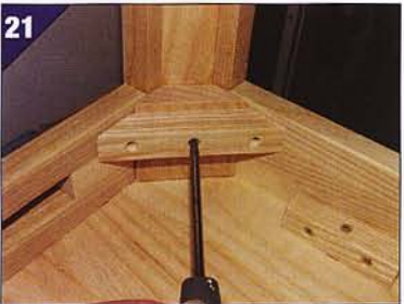
Attach the second leg support
