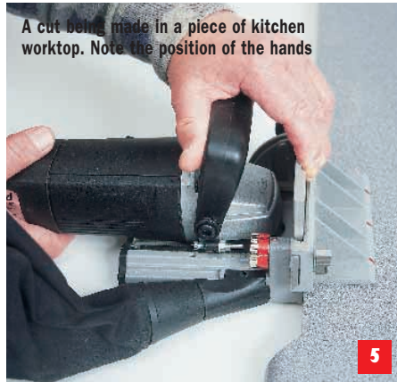
A board being slotted with the jointer base running on the worktable surface
