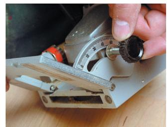
There is no height adjustment on the flip fence, although it's sturdy
