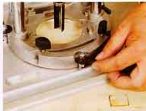
Recesses on the base allow you to clip the router in and out of the Trend PRT table (Clips £22.92)
