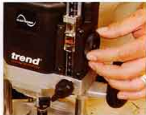
Standard height adjustments can still be made using the dial and plunge post
