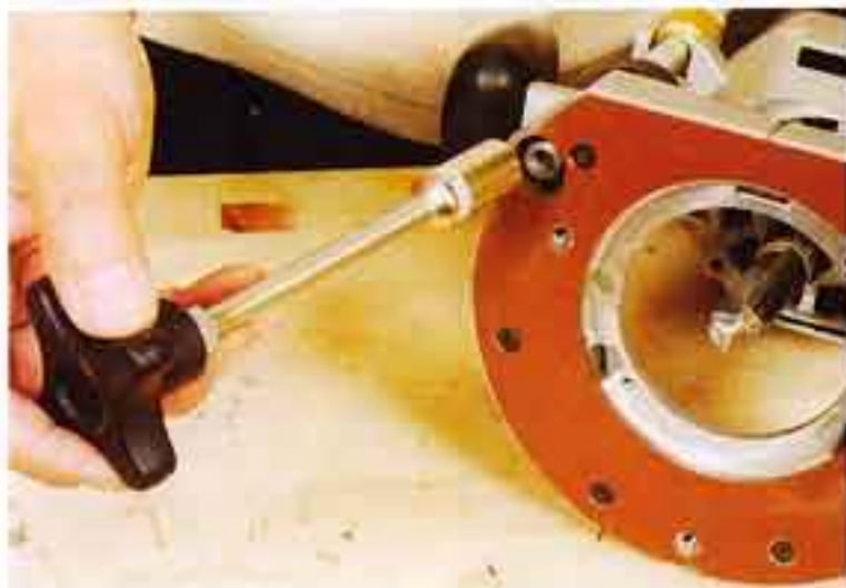
The fine height adjuster will also alter the setting through the router base
