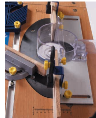
Fence assembly with dust extraction and cutter guard
