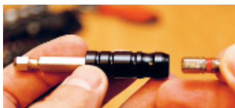
▲ With the black sleeve forwards the standard 6.3mm hex bits are held
