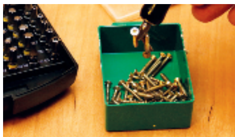
▲ The SB3 bit holder magnet works well enough with a short bit fitted...
