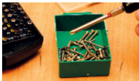
▲ ...but with the longer bits there's no magnetism at all through the bit
