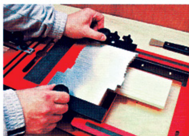
▲ Once the comb is set it is flipped to act as a template
